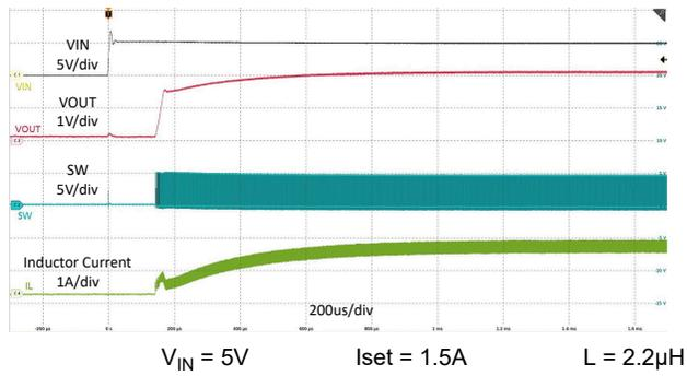
**Figure 8-8. VIN Control Start Up with Load**
