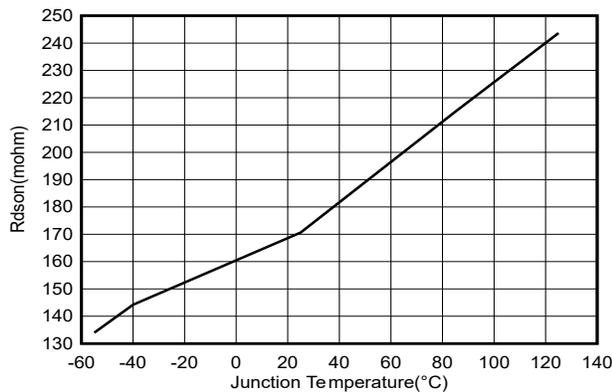
Figure 6-5. Low-Side FET On Resistance vs Junction Temperature
