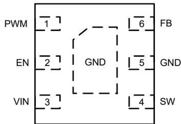
Figure 5-1. DRV Package 6-Pin WSON Top View
