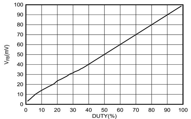
Figure 6-6. PWM duty cycle vs FB voltage
