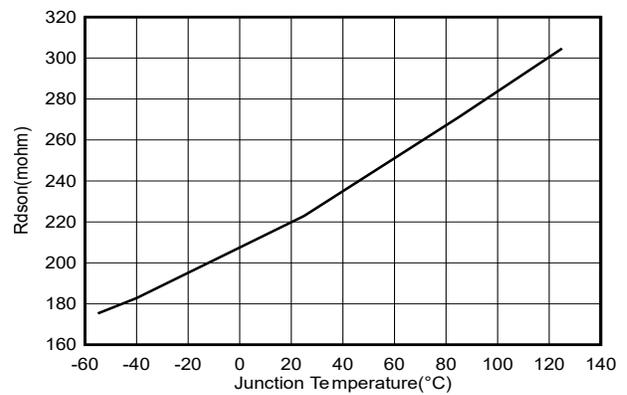
Figure 6-4. High-Side FET On Resistance vs Junction Temperature
