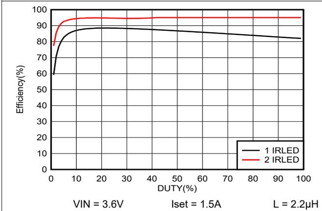
**Figure 8-4. Output Efficiency at 3.6V Input Voltage**
