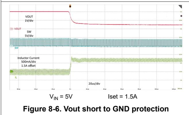
**Figure 8-6. Vout short to GND protection**
