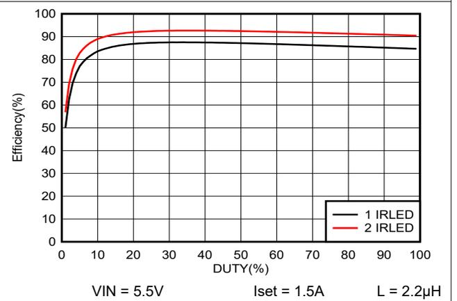
**Figure 8-5. Output Efficiency at 5.5V Input Voltage**
