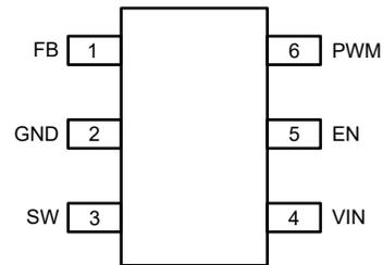
Figure 5-2. DRL Package 6-Pin SOT563 Top View
