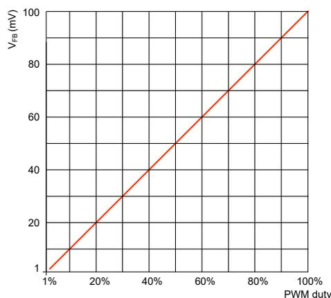
**Figure 7-2. FB voltage with PWM duty cycle**
